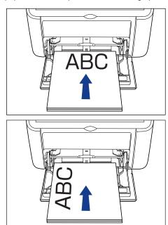
5 Slide the paper guides to fit both sides of the stack.
